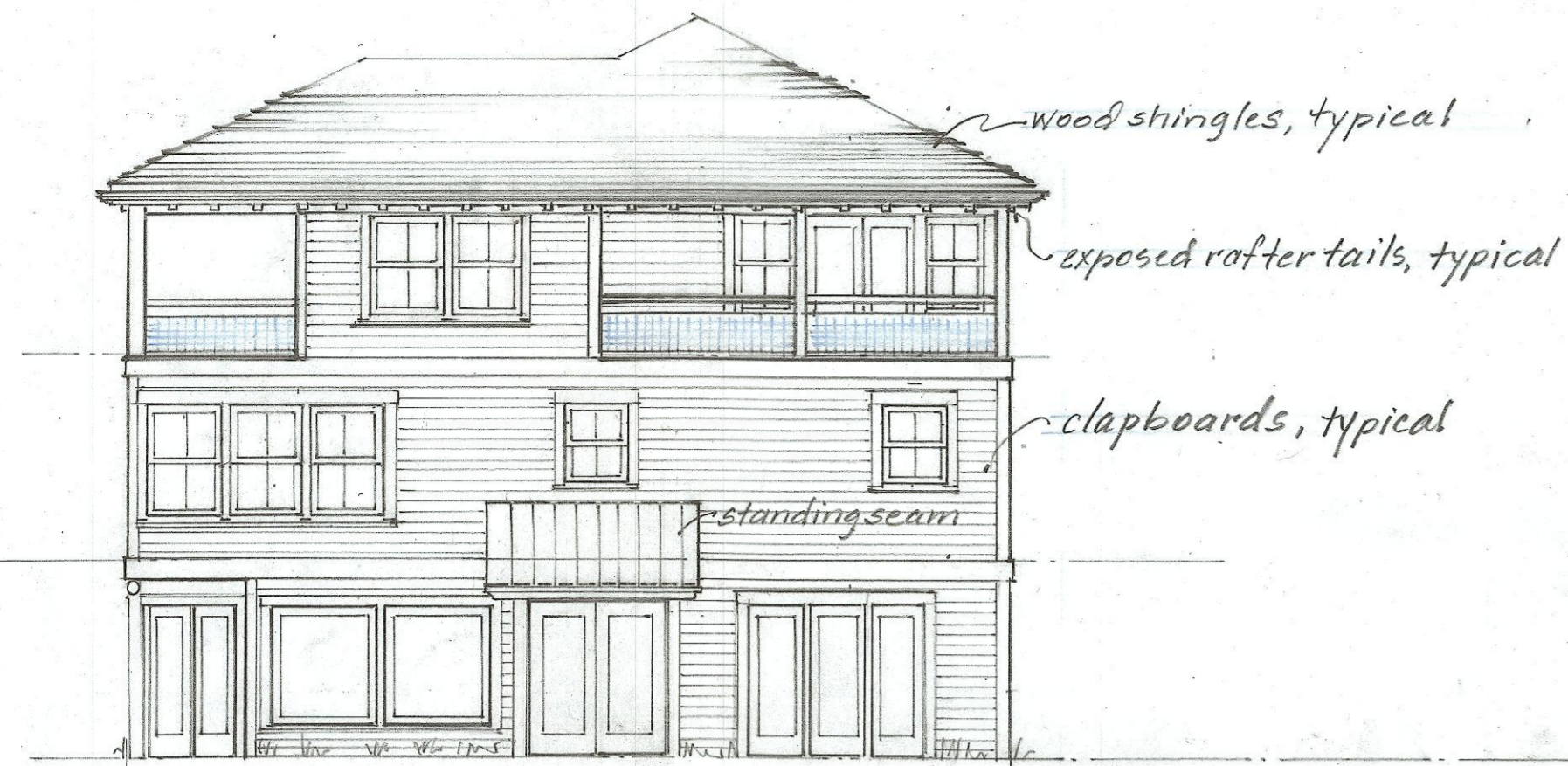
EAST ELEVATION UNITS C-4 R-11 & R-10 SCALE: 1/8" = 1'-0" 01.04.2021 01.05.2021 01.10.2021
