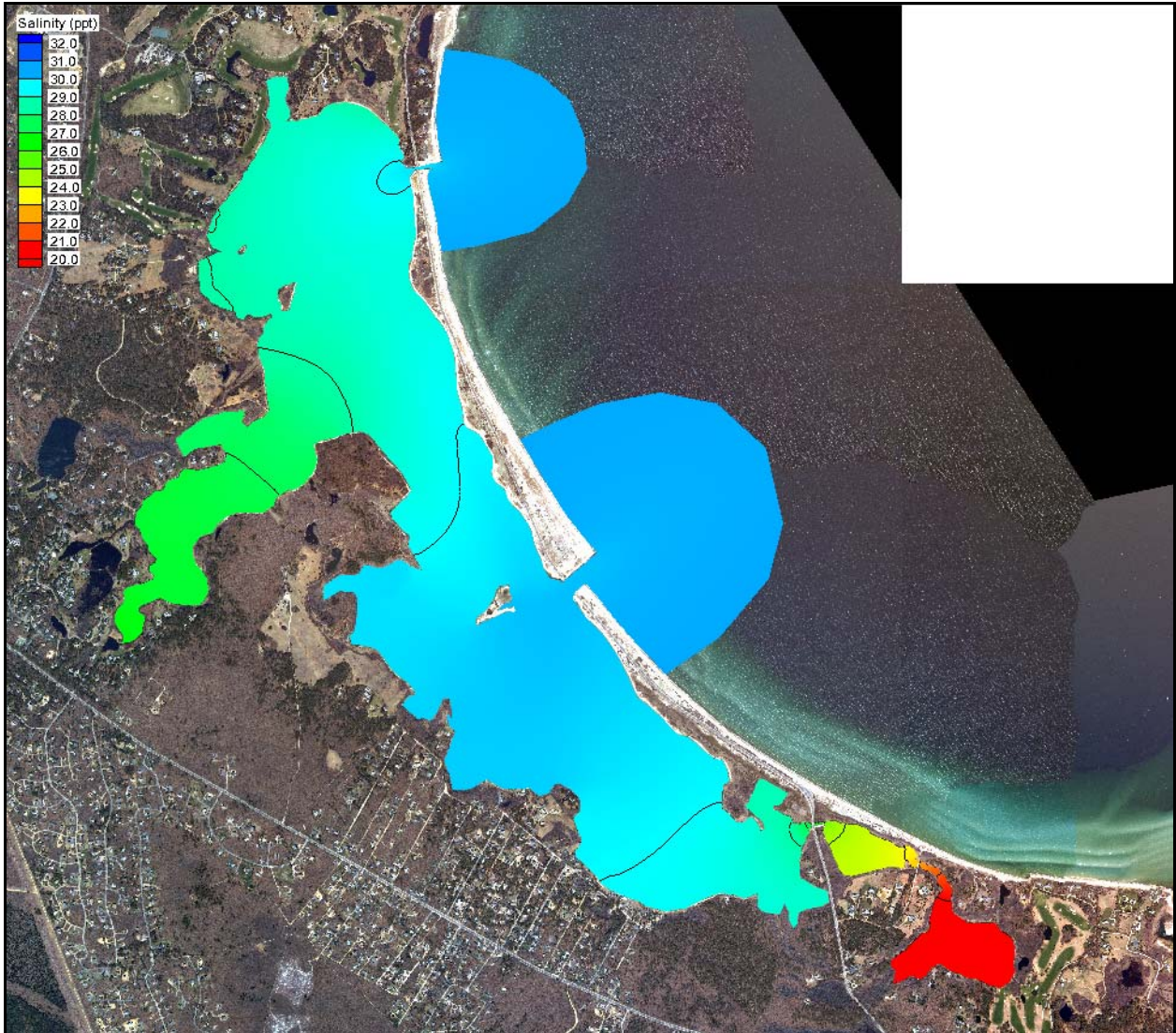
Figure VI-6. Contour plots of modeled salinity (ppt) in Sengekontacket Pond System.
