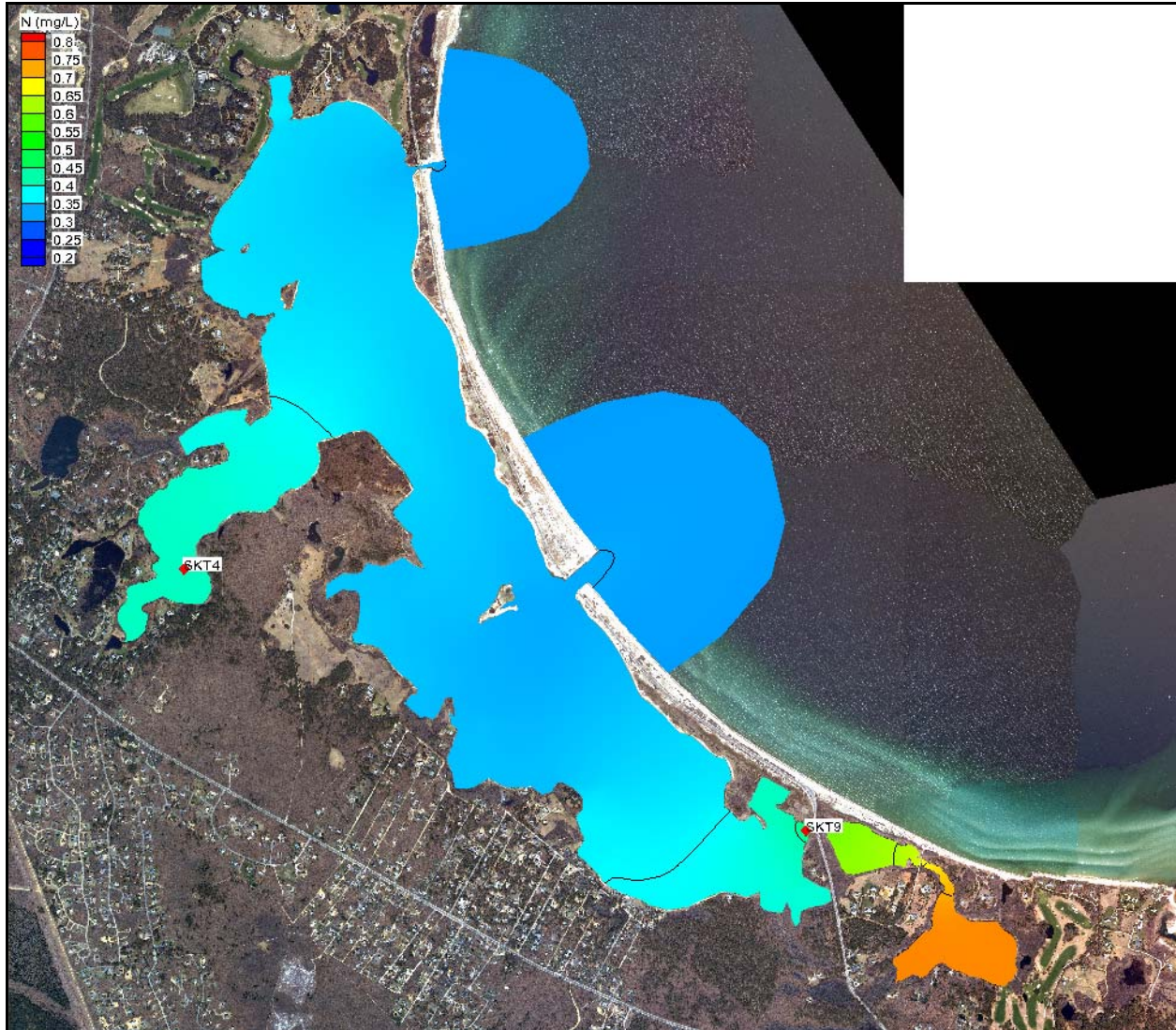
Figure VI-7. Contour plots of modeled total nitrogen concentrations (mg/L) in Sengekontacket Pond System, for projected build-out loading conditions, and bathymetry. The approximate locations of the sentinel threshold stations for Sengekontacket Pond System (SKT-4 and SKT-9) are shown.
