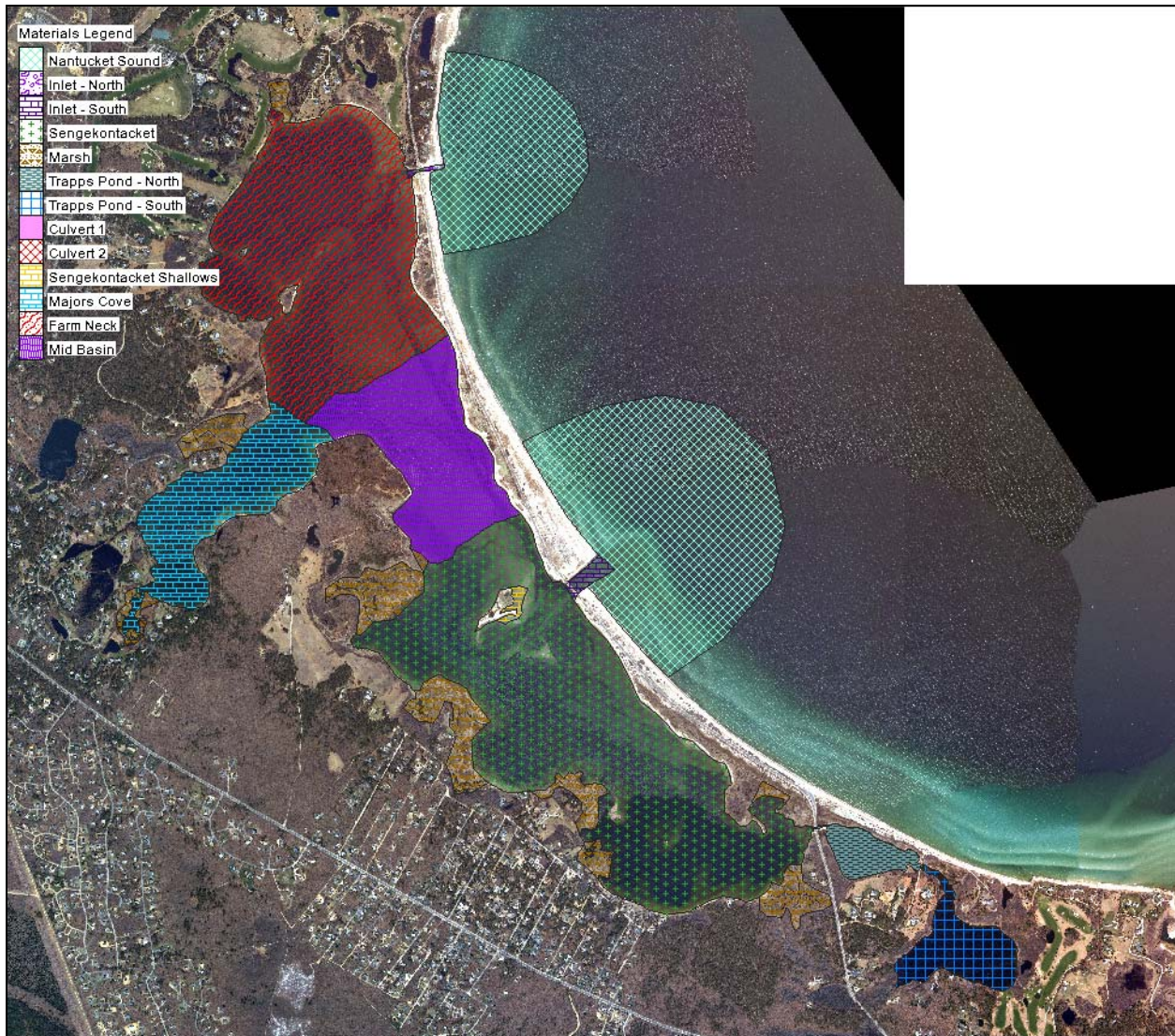
Figure VI-2. Map of Sengekontacket Pond water quality model longitudinal dispersion coefficients. Color patterns designate the different areas used to vary model dispersion coefficient values.
