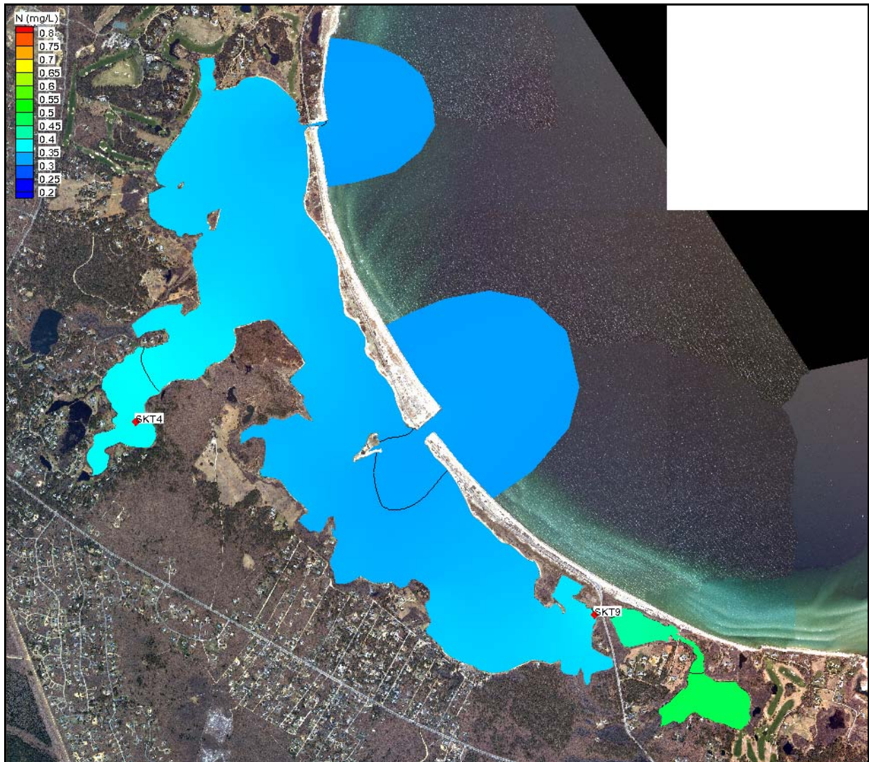
Figure VIII-1. Contour plot of modeled average total nitrogen concentrations (mg/L) in Sengekontacket Pond system, for threshold conditions (0.35 mg/L at water quality monitoring stations SKT-4 and SKT-9), to restore eelgrass habitat within Majors Cove/Sengekontacket Pond and to improve eelgrass habitat within Trapps Pond. The approximate locations of the sentinel threshold stations for Sengekontacket Pond (SKT-4 and SKT-9) are shown. There is no baseline water quality station within Trapps Pond.
