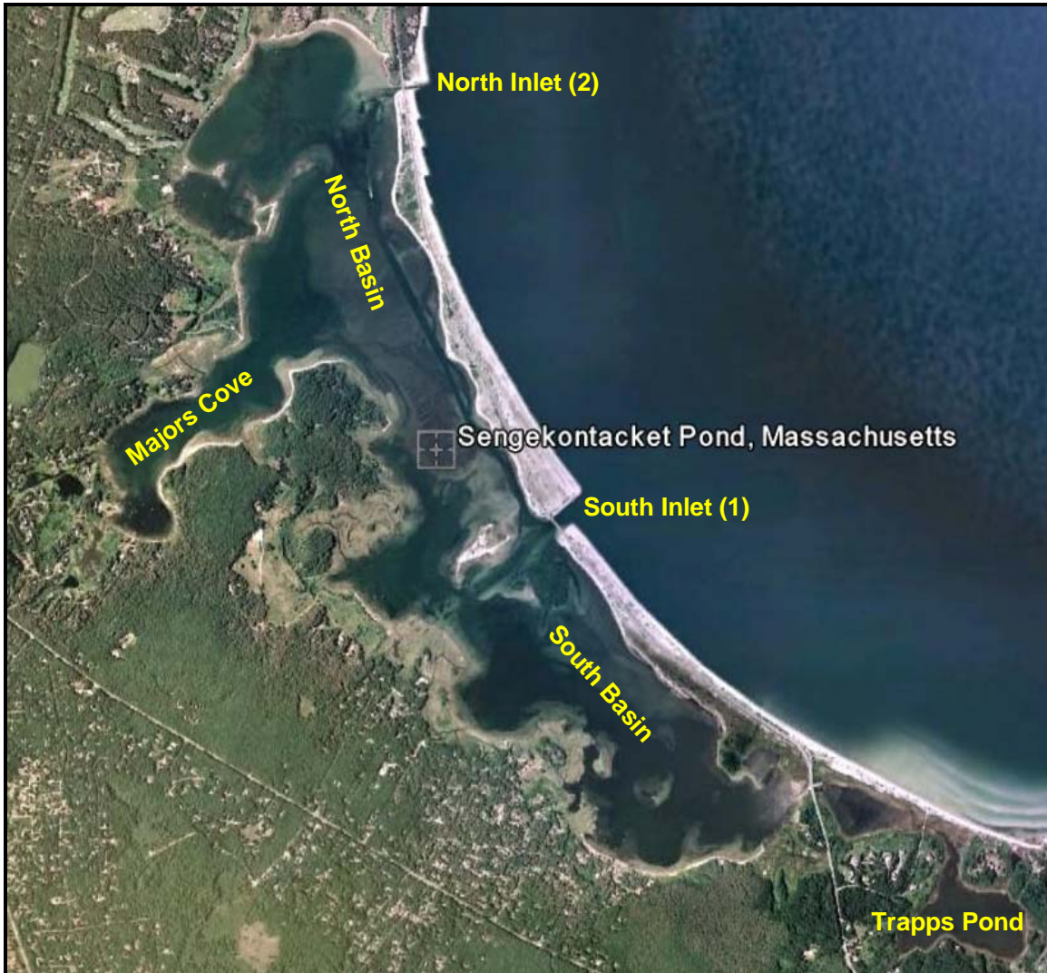
Figure I-2. Study region for the Massachusetts Estuaries Project analysis of the Sengekontacket Pond Embayment System. Tidal waters enter the Pond through two inlets passing through the barrier beach and allowing tidal exchange with waters from Vineyard / Nantucket Sound. Freshwaters enter from the watershed primarily through direct groundwater discharge as there are no significant surface water inflows to this system.
