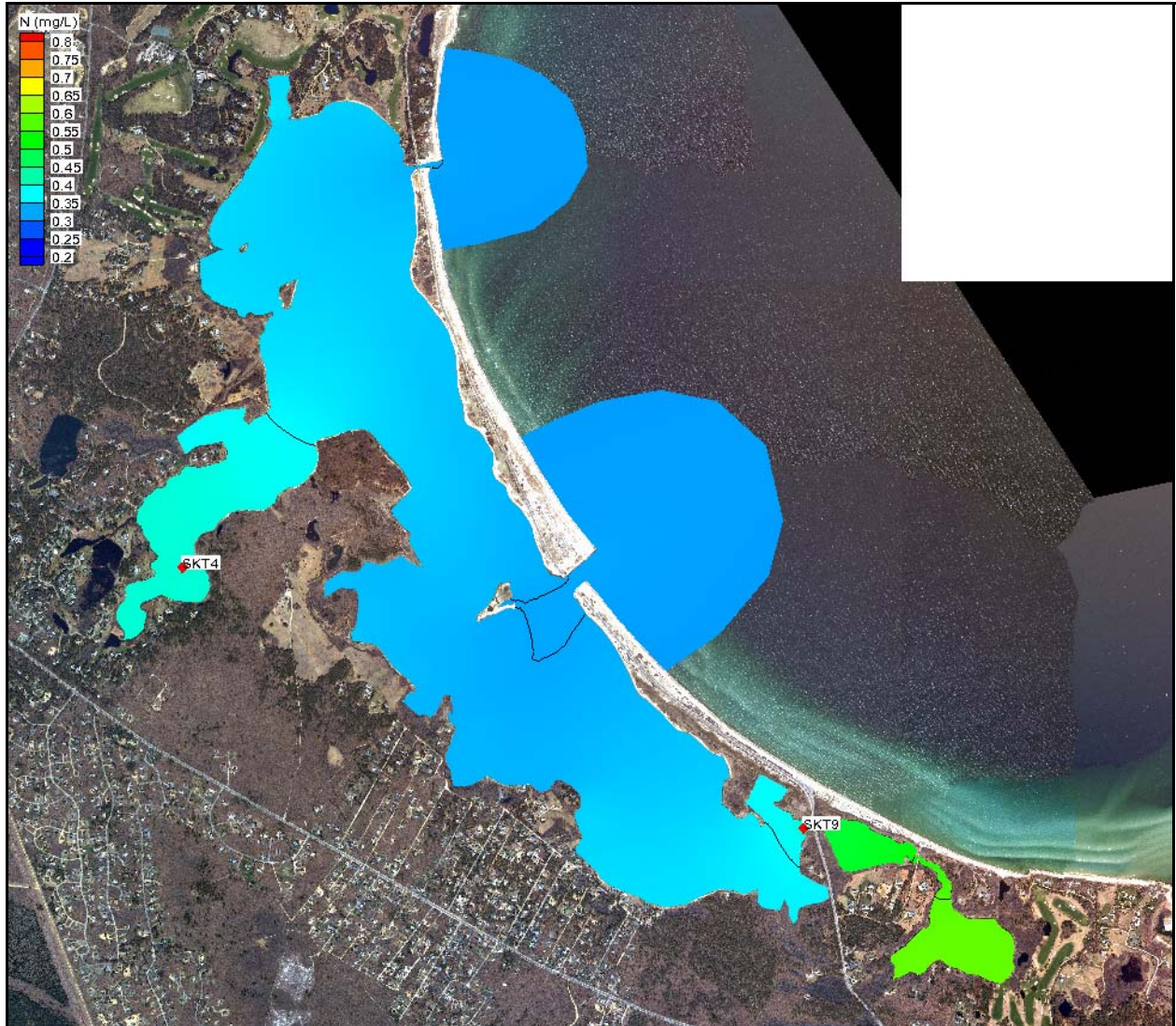
Figure VI-4. Contour plots of average total nitrogen concentrations from results of the present conditions loading scenario, for Sengokontacket Pond System. The approximate locations of the sentinel threshold stations for Sengokontacket Pond System (SKT-4 and SKT-9) are shown.
