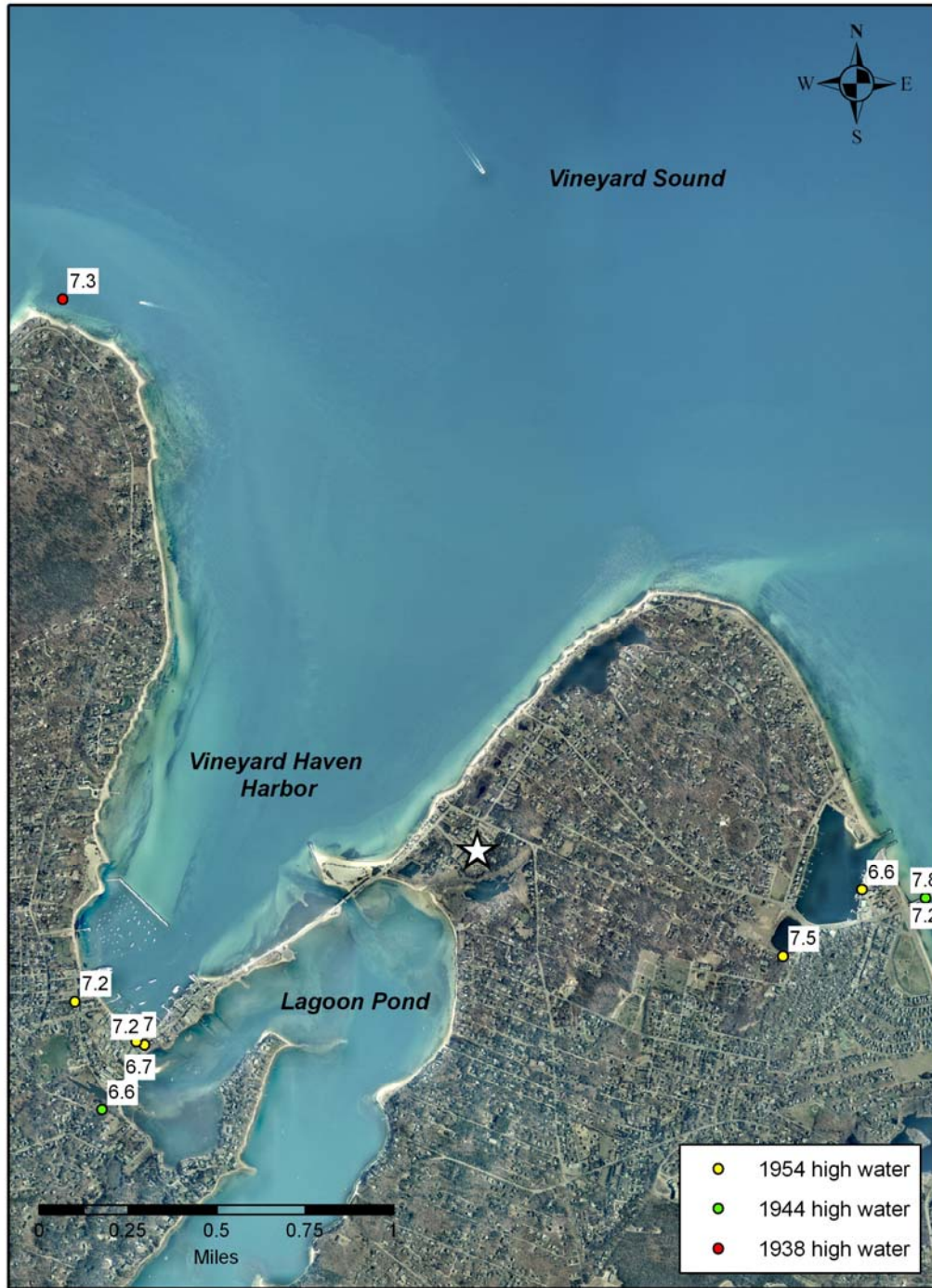
Figure 7. Map showing storm surge high water measurements for the 1938, 1944, and 1954 hurricanes (recorded in ft above NGVD).
