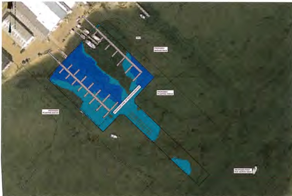
Figure 1: Image obtained from the hydrographic survey sketch plan that shows the depth of sediment that needs to be dredged to reach the design grade of -4' MLW (5.29 NAVD88). Note the contours shown are on NAVD88 Vertical Datum.
