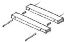
'Flex' Construction. Assembled with stainless steel rod shipped in semi-rigid sections that flex in all directions, contouring to almost any surface, even turning slightly to the left or right for curves. The sections quickly & easily bolt together.
