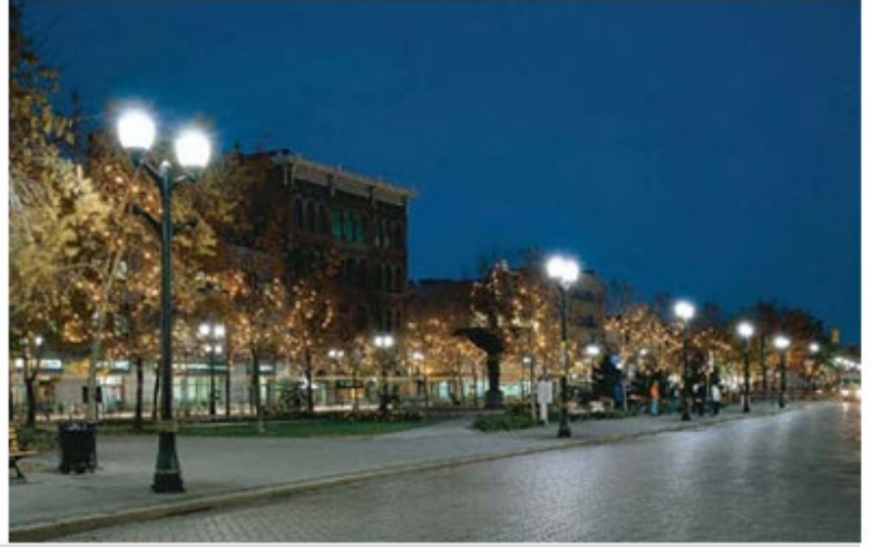
Pedestrian scale lighting is shorter and slightly dimmer than streetlights. Source: FHWA. Source: https://safety.fhwa.dot.gov/roadway_dept/night_visib/lighting_hanbook/#fig46
