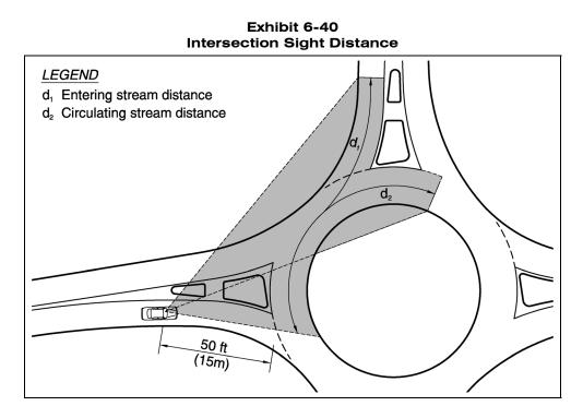
Intersection sight distance should be measured using an assumed drivers eye height of 3.5 ft (1,080 mm) and an assumed height of object of 3.5 ft (1,080 mm) in accordance with the fourth edition of the AASHTO publication, "A Policy on Geometric Design of Highways and Streets" (Green Book).
