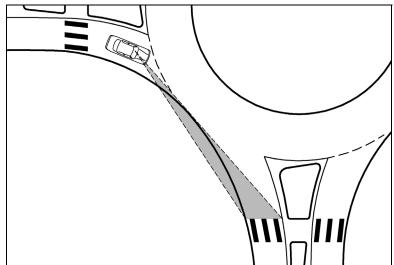
Stopping sight distance should be measured using an assumed drivers eye height of 3.5 ft (1,080 mm) and an assumed height of object of 2 ft (600 mm) in accordance with the fourth edition of the AASHTO publication, "A Policy on Geometric Design of Highways and Streets" (Green Book).
