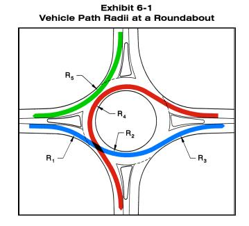
The fastest path is drawn assuming a vehicles starts at the left-hand edge of the approach lane, moves to the right side as it enters the roundabouts, cuts to the left side of the circulatory roadway, then moves back to the right side at the exit, and completes its move at the left-hand side of the departure lane. The centerline of the vehicle path is drawn using the following minimum offset distances:
