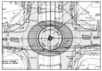
provided, varying in width from about 6.5 ft (2 m) to about 16.4 ft (5 m). The outside curb around the roundabout is a KDOT Type I; the inside curb is a KDOT Type III. The curb around the splitter island is a 9-in (230-mm) wide KDOT protection curb, modified to 6 in (150 mm) in height. The pavement in the roundabout is asphalt, with a 9-in (225-mm) base and 1-in (25-mm) surface course.
