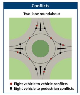
**Figure 1:** Eight Vehicle Conflict Points *Source: FHWA Roundabouts: An Informational Guide*
