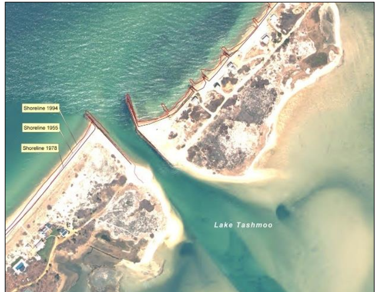
Shoreline change in the area of Lake Tashmoo showing shorelines from 1955, 1978 and 1994 and 1978 (CZM data)
