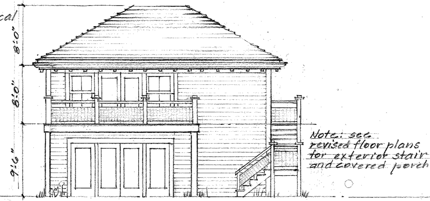
EAST ELEVATION UNITS C-3 & R-9 SCALE: 1/8" = 1'-0" 01.04.2021 01.05.2021 01.10.2021
