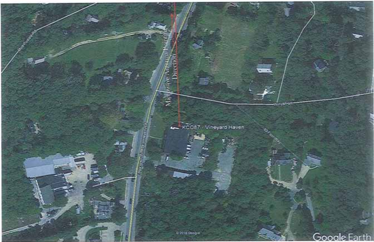
Figure 1 - Aerial Image Showing Location/Azimuth of Microwave Antennas
