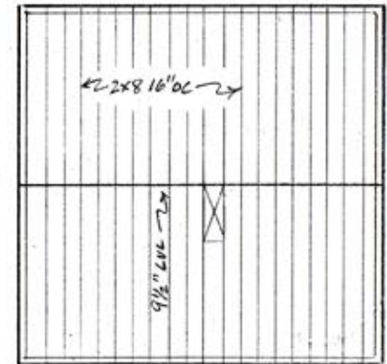
2ND FLOOR CEILING JOISTS
