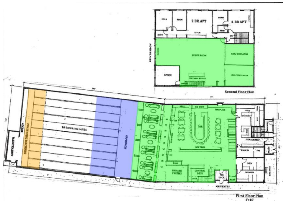
Figure 1: Proposed Layout: Green areas: Possible Music and People Activity Sound Generation, Purple Area: Bowling Ball impact on the lane/floor, Orange Area: Pinsetter and Ball Impact Pins and Pit-Cushion. All highlighted areas are high noise level spaces, Orange being the likely location for highest noise level, although music in the Green areas could be as loud depending on settings.
