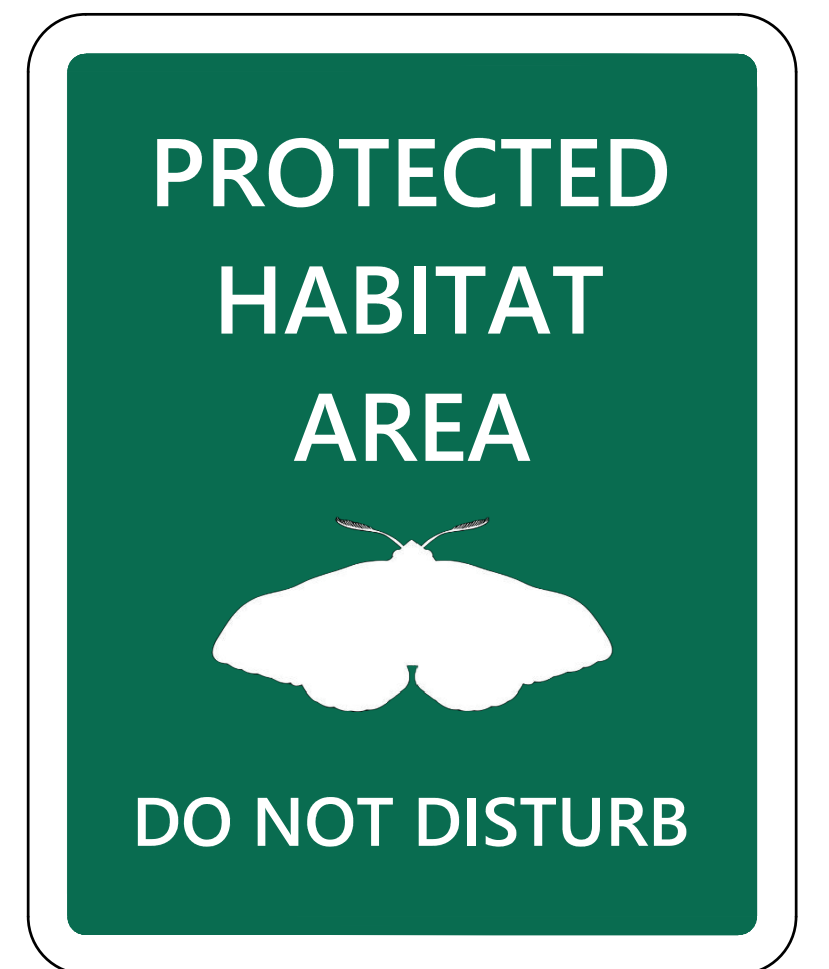
NOTE: WEATHER RESISTANT 8" x 10" ALUMINUM SIGN. 3/8" HOLES DRILLED AT TOP & BOTTOM CENTER. INSTALL ON 4"x4" WOOD POST. PROTECTED HABITAT SIGN SCALE: 1:2
