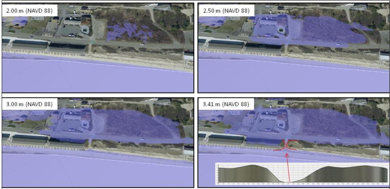
Figure 5. Draped aerial photograph over Lidar surface in North Truro. Blue areas are horizontal plane created in Fledermaus at increasing elevation. Lower right is example of a storm-tide pathway with accompanying profile. These images were generated before field work to identify potential STPs (image taken from Borrelli, et al. 2017).
