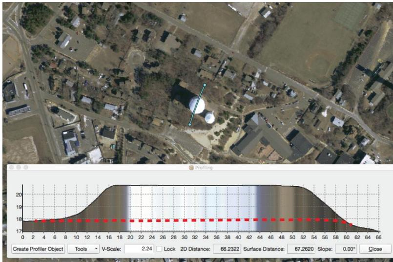
Figure 4. Example of ‘pull up’ near a water tower in Provincetown. Dotted red line is more representative of elevations at the water tower. Blue line in image is location in profile. Profile units = meters (Vert. NAVD88, Hor. NAD83), image taken from Borrelli, et al. 2017.
