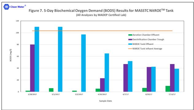
Referring to Figure 6, total suspended solids levels were consistently maintained near 10 mg/l and lower with an average influent level slightly above 50 mg/l. Figure 7 shows significant  $BOD_5$  reduction as evidenced with aeration chamber effluent concentrations less than 10 mg/l with an influent average slightly more than 100 mg/l. The cited  $BOD_5$  increases measured in the denitrification chamber trough
