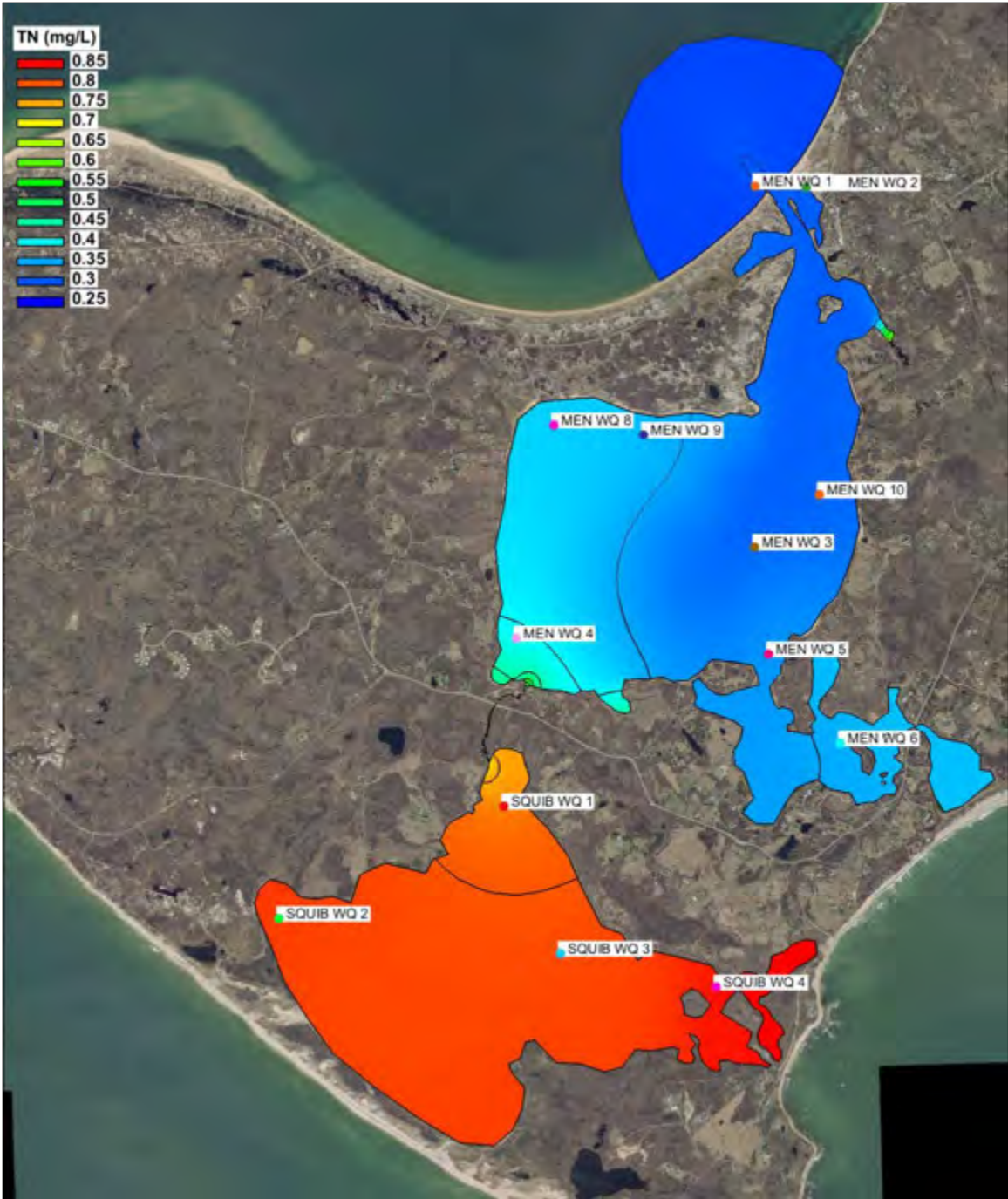
Figure VI-8. Contour plot of modeled total nitrogen concentrations (mg/L) in the Menemsha and Squibnocket Ponds system, for projected build-out scenario loading conditions.
