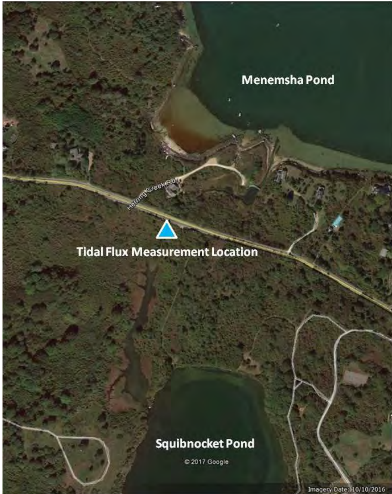
Figure IV-11. Location of tide gauge deployed in Herring Creek to measure stage during the 08/02/10 (1 day off the quarter moon, neap tide) and 08/15/10 (1 day off the quarter moon, neap tide) tidal sampling events. During the 2010 tidal flux studies a stage recorder was positioned up-gradient of the State Road culvert.
