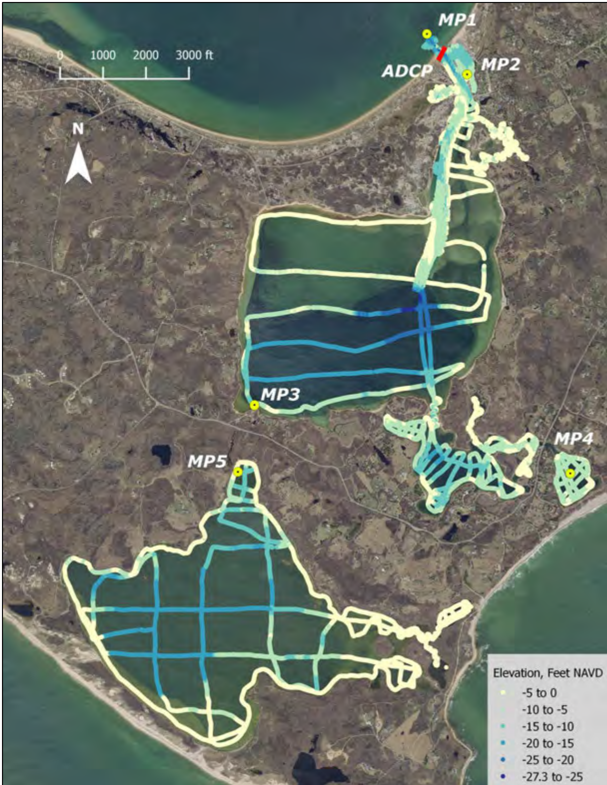
Figure V-2. Boat lines from the 2013 USACE and 2015 SMAST bathymetry surveys of the Menemsha-Squibnocket Pond Embayment System. Yellow markers show the locations of the tide recorders deployed for this study. The cross-channel transect followed during the ADCP survey of tidal velocities (at the inlet) is indicated using the solid red line.
