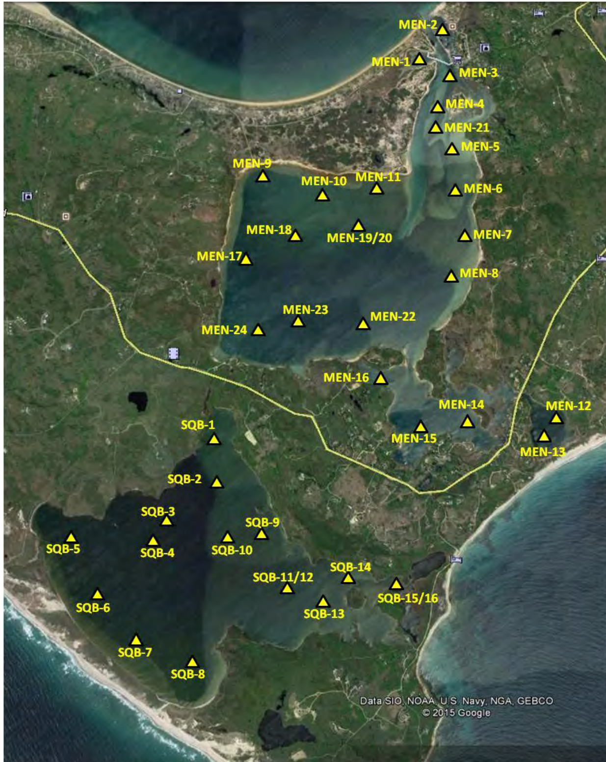
Figure IV-12. Menemsha-Squibnocket Pond Embayment System sediment sampling sites (yellow symbols) for determination of sediment-water column exchange rates. Numbers are for reference to station identifications listed below and in Table IV-5.
